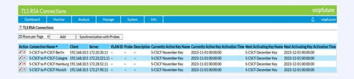
The keys can be added on the new TLS RSA Keys and Add/Edit TLS RSA Key pages. On the new TLS RSA Connections and TLS RSA Connection pages the different private keys can then be assigned to different SBC connections. and It is also possible to set an automatic activation time, to ensure keys are changed at the same time as by the monitored SBCs will activate them can be scheduled.
