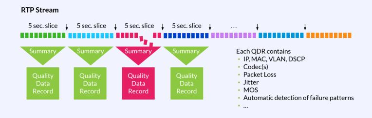
Indicators enable effective root cause analysis, as they automatically identify QDRs that suffered from specific impairment types, such as network overload conditions. The key to this is Voipfuture's
